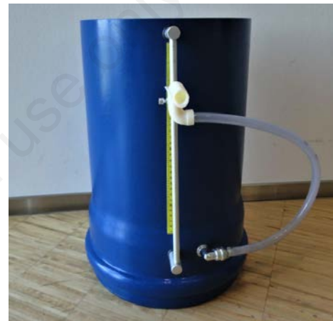
Figure 2. Water plethysmograph with variable overflow.
