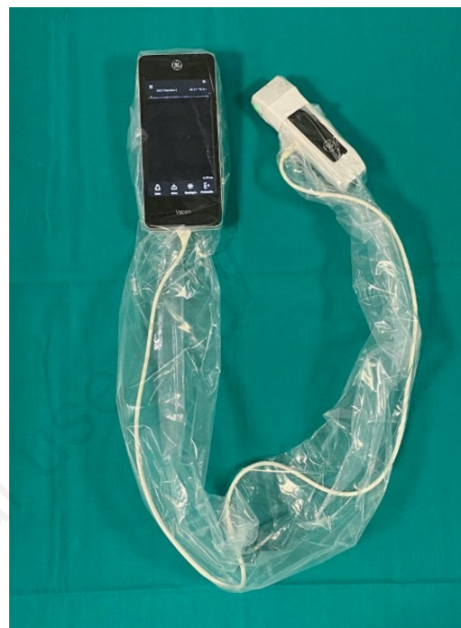
Figure 1. Both the pocket-sized display unit and the probe of the handheld ultrasound system are enclosed within a single sterile plastic sheath.
