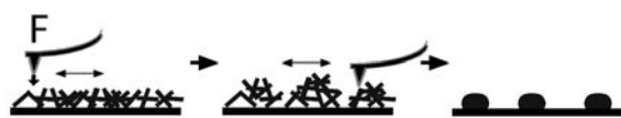
Figure 1. Schematic drawing of the patterning mechanism of rotaxane thin films upon the mechanical perturbation of an AFM tip.
