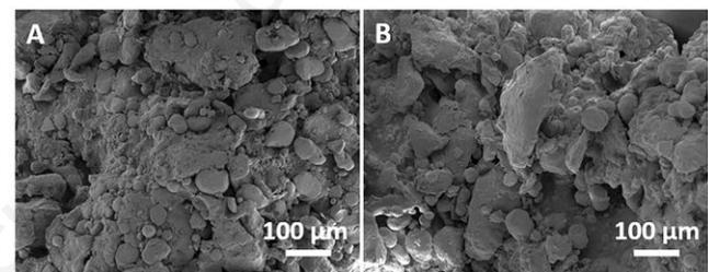
**Figure 3.** SEM micrographs of PCL particles partially melted on DO (A) and RD (B) scaffolds surface.
