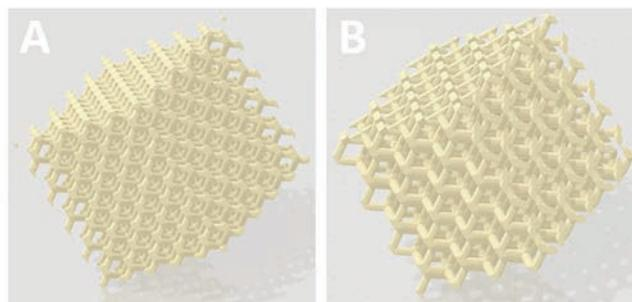
**Figure 1.** PCL/HA lattice scaffolds with diamond (A) and rhombic dodecahedron (B) elementary unit cells.
