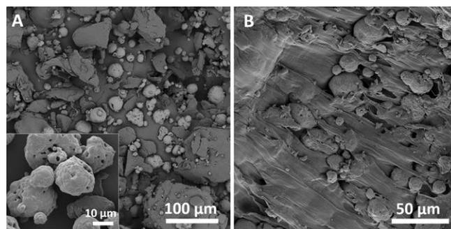
**Figure 2.** Backscattered SEM micrograph of (A) PCL/HA (30 wt.%) powder mixture and (B) HA particles in PCL matrix of a manufactured scaffold.
