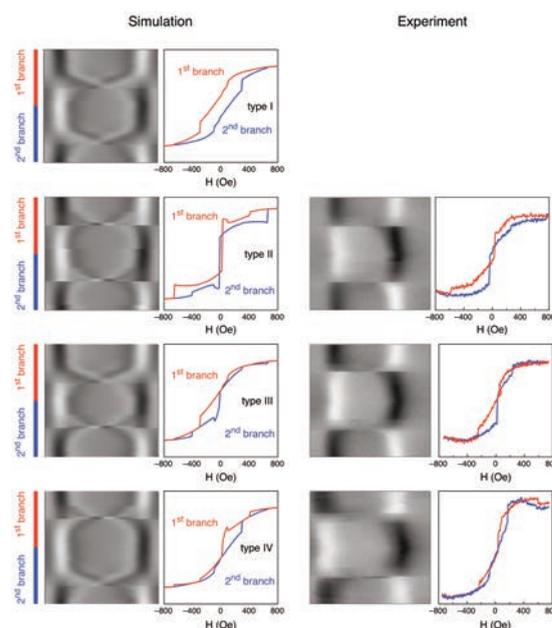
**Figure 1.** Comparison between simulated (left) and experimental (right) MFM images, and corresponding local hysteresis loops, of a  $\text{Ni}_{80}\text{Fe}_{20}$  square dot submitted to an in-plane magnetic field.
