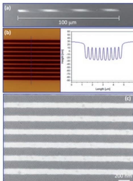
**Figure 1.** (a) SEM image of the entire lateral standard. (b) AFM analysis of the DBC disposition inside the periodic grating. (c) SEM micrograph representing the directed self-assembly of DBC inside the periodic gratings.
