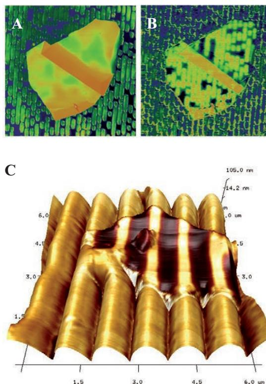
**Figure 2.** (A) Topography image of a graphitic flake on deposited on top of the patterned COC substrate. (B) UFM image of the same graphitic flake showing a contrast due to its subsurface imaging capability. (C) UFM image superimposed to a topographic one of a MoS<sub>2</sub> flake: also in this case UFM demonstrates its subsurface sensitivity showing the presence of grooves under the 2D-material flake. The topography images were both obtained with TM-AFM.
