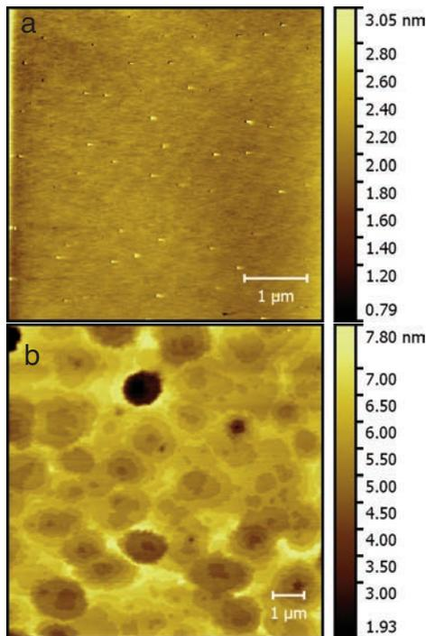
**Figure 1.** AFM images of the same  $1.6 \times 10^{20} \text{ cm}^{-3}$  Al+ implanted 4H-SiC sample before (a) and after (b) the  $1950^\circ\text{C}/12 \text{ min}$  post implantation annealing with C-cap (removed before AFM measurements).
