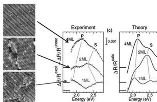
Figure 1. STM images (50 x 50 Å<sup>2</sup>) of the (105) surface for increasing coverage  $\theta$  of Ge and corresponding measured RAS spectra (central panel) for the same coverage values. Computed RAS spectra are also compared (right panel). Lines are a guide for the eye.
