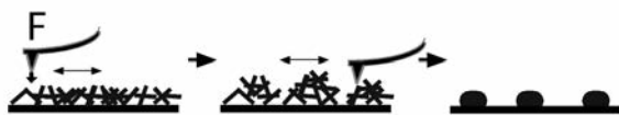
Figure 1. Schematic drawing of the patterning mechanism of rotaxane thin films upon the mechanical perturbation of an AFM tip.
