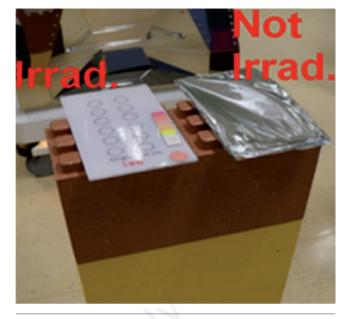
Figure 1. The areas within the circumferences were contaminated with the strains used during the test. The surface of the material not irradiated was wrapped 3 times in aluminum foil for protection. The surface of the material irradiated was exposed to UV-C light.
