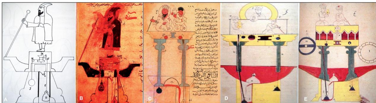
has been drained into the tank, the float rises and the “G” reel spins. In accordance with the spinning of the reel, the monk and its rod spin in a way that shows the amount of blood taken. The rod in the hand of the monk reaches the first sign once 1 dirham (dirham = 3.207 gr) of blood has been collected in the tank (5).
