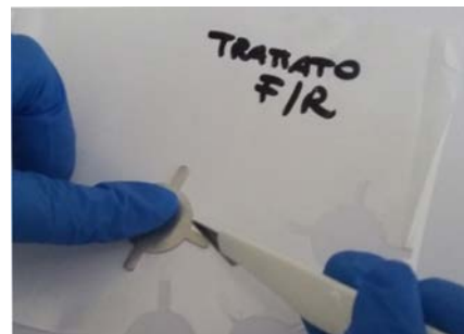
Figure 1. Cutting of flexible packaging materials with a steel mold.
