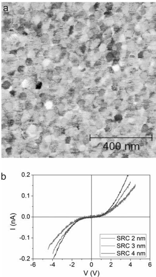
**Figure 1. (a) C-AFM performed on sample with SRC layer thickness of 4 nm. (b) Local IV measured with AFM for different SRC layer thickness. Each curve is the average of 10 measurements taken in different positions on the sample surface.**
