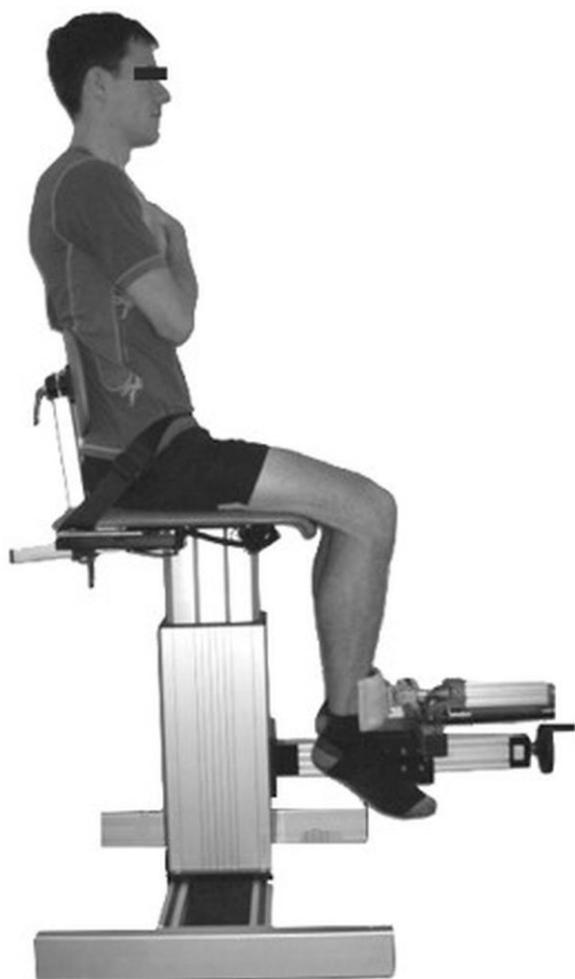
**Fig 1.** Measuring system "SeBit knee" for the detection of Adaptive Force (AF) of the quadriceps femoris muscle.
