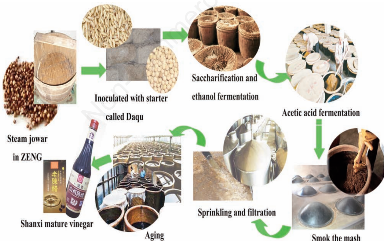
Figure 1. Flow sheet for Shanxi aged vinegar production. The primary materials are jowar and Daqu ; the process may be divided into five mainly processes, namely starter preparation, fermentation, smoking, sprinkling and aging. The whole production period lasts one year or longer.
